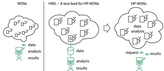
Fig. 1. The HWL test-bed enables the development and analysis of applications for HP-WSN.
