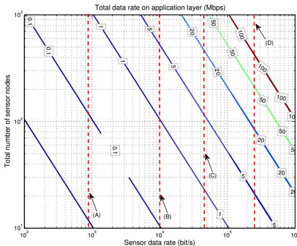
Fig. 2. Data rate on application layer (Mbps) depends on the number of sensor nodes and the sensor data rate.
